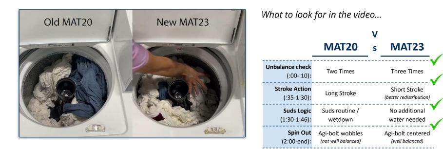
Better balancing = Less energy dissipated through suspension, motor, belts, etc
